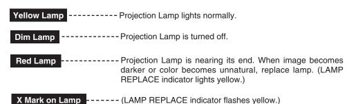
Projection lamp is defective or fails to be turned on. Restart a projector on, and make sure lamp is on. If this mark still appears, replace lamp corresponding with number marked X.
